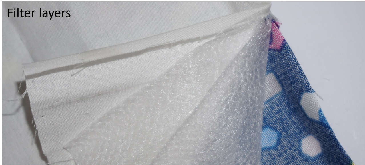
Style Z (tied) Filter layers 2x thin (30 gsm)
